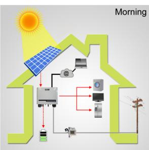
Energy produced by the PV system is used to optimize self-consumption. The excess energy is used to recharge the batteries.
